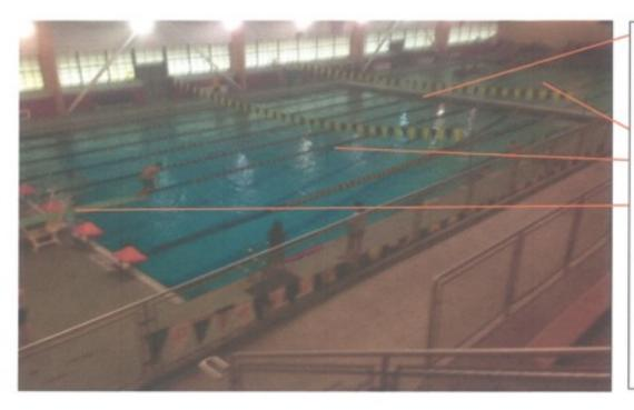
Bulkhead: A bridge that can be inflated and repositioned to create two swim areas (as pictured) which is a total of 16 lanes, or if positioned against shallow end wall, one large 8 lane, 50 meter pool.
